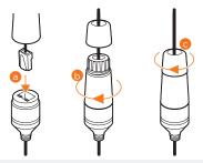
NOTE: When using the waterproof cap, crimp the RJ45 connector after passing the cable through the waterproof cap.
