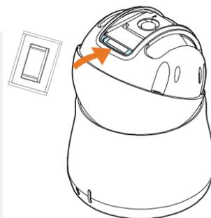
**WARNING:** It is highly recommended that you install the moisture absorber when mounting the camera. The moisture absorber prevents moisture from being captured inside the camera's housing, which may cause image performance issues and damage the camera.
