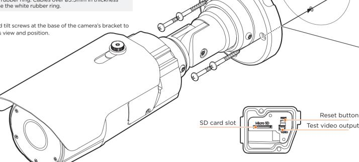
**Resetting the camera:** To reset the camera, press the reset button on the external control panel for five (5) second. The system will initiate a camera-wide reset of all the settings. including network settings.
