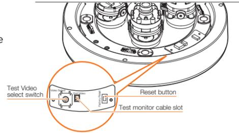
**Resetting the camera:** To reset the camera, use the tip of a paper clip or a pencil and press the reset button. Pressing the button for five (5) seconds will initiate a camera-wide reset of all the settings, including network settings.
