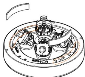
**NOTE:** The camera will generate enough heat to dry moisture during operation. In most cases it will not need the moisture absorber for more than the first day. In cases where the camera can experience a moisture issue, users must keep the moisture absorber in the camera. The moisture absorber has an approximately 6-month life cycle, varying depending on the environment.
