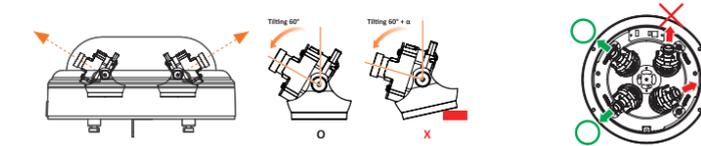
**NOTE:** When installing the camera, align the sensor module's direction as shown in the diagram on the left and fix the dome cover carefully. Image distortion may occur if the modules are not installed correctly.
