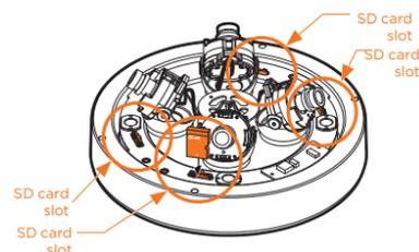
**NOTE:** The camera can accommodate up to 4 SD card slots. See the diagram above for position.
