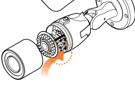
**STEP 2 - CABLING THE CAMERA TO EXTERNAL DEVICES**
