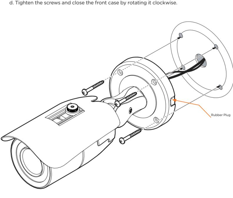
**NOTE:** Based on the installation environment, remove the rubber plug on the side of the camera's bracket and use the gap as a cable guide to prevent cables from getting caught between the camera and the mounting surface, which can cause damage to the cables and prevent the camera from mounting flush with the mounting surface.
