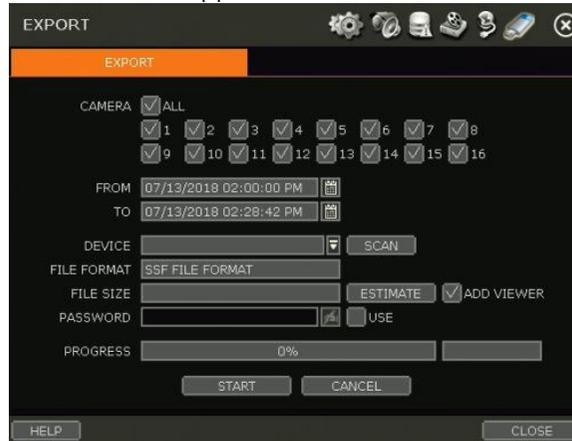
3. Connect an appropriate USB memory drive and press [SCAN] to recognize it before starting the backup process.
