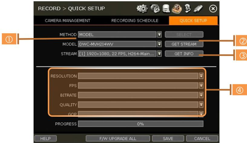
1. Select the model or camera multi-select to setup. When selecting the 'Model' method, all cameras with the same model's name will be selected.
