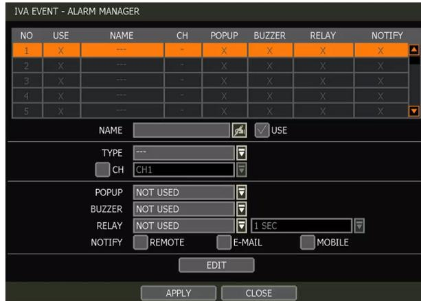
If the user checks 'USE', the setting window is activated and the user can set the event alarm name, type, and notification type (pop-up, buzzer, relay, etc.).
