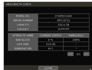
**WARNING** To achieve high-level system stability, a warning message of elevated temperature will pop up when the temperature inside the system exceeds the best range. This problem may be driven by the malfunction of ventilation fans. Inspect if the cooling fan is properly working, or temperature around the system is meticulously kept.
