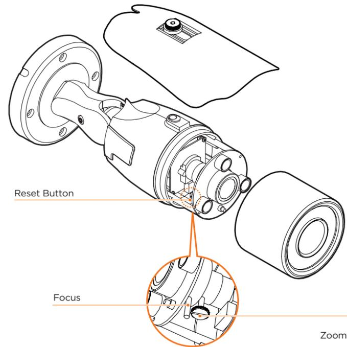
**Resetting the camera:** To reset the camera, use the tip of a paper clip or a pencil and press the reset button. Pressing the button for five (5) seconds will initiate a camera-wide reset of all the settings, including network settings.
