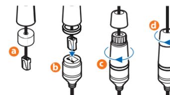
**NOTE:** To ensure moisture seal, make sure the o-ring is in place between a and b. In extreme environments use of an outdoor rated sealer is recommended.
