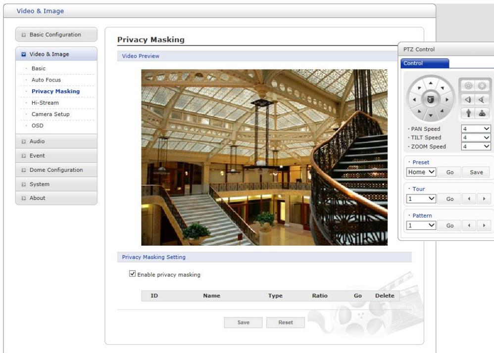
The privacy masking function allows you to mask parts of the video image to be transmitted. You can set up to sixteen privacy masks. Only up to 8 privacy masks can be displayed on one screen.
