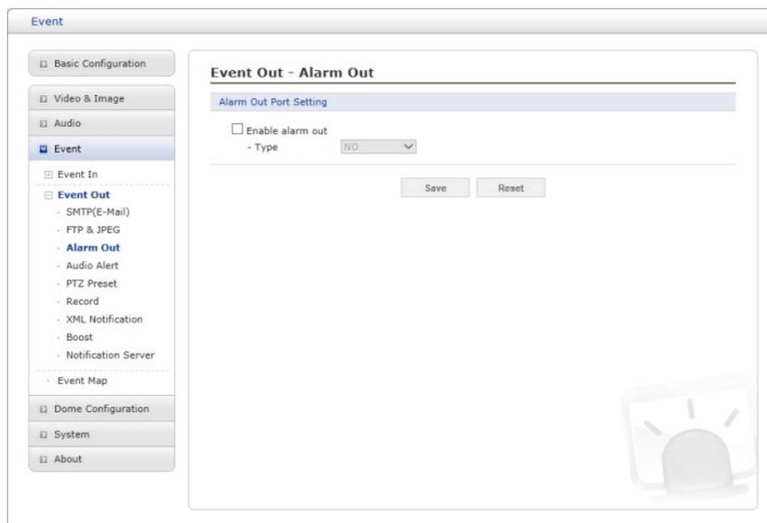
When the camera detects an event, it can control external equipment connected to its alarm output port.
