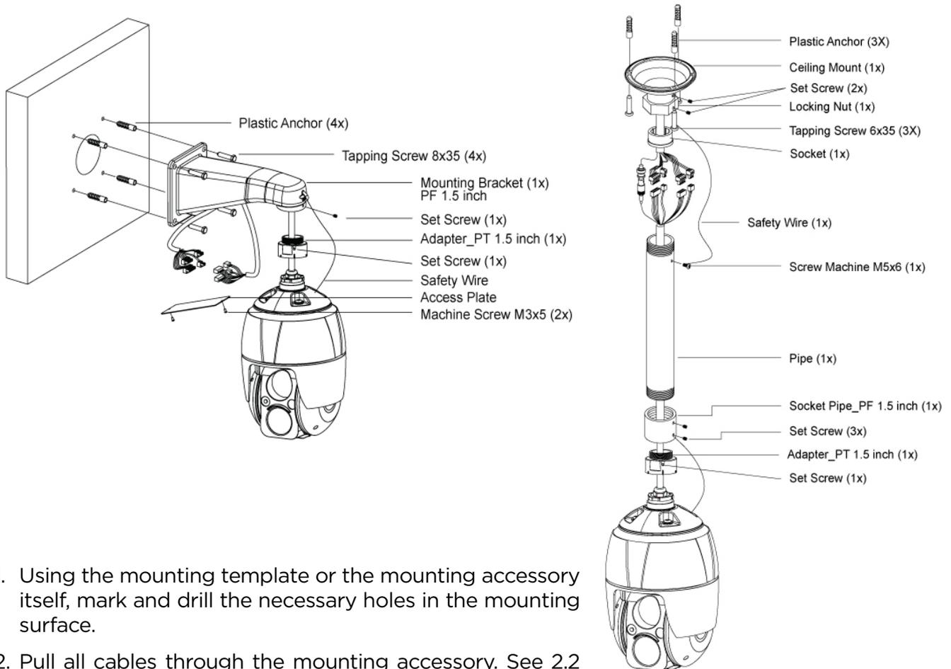
1. Using the mounting template or the mounting accessory itself, mark and drill the necessary holes in the mounting surface.
