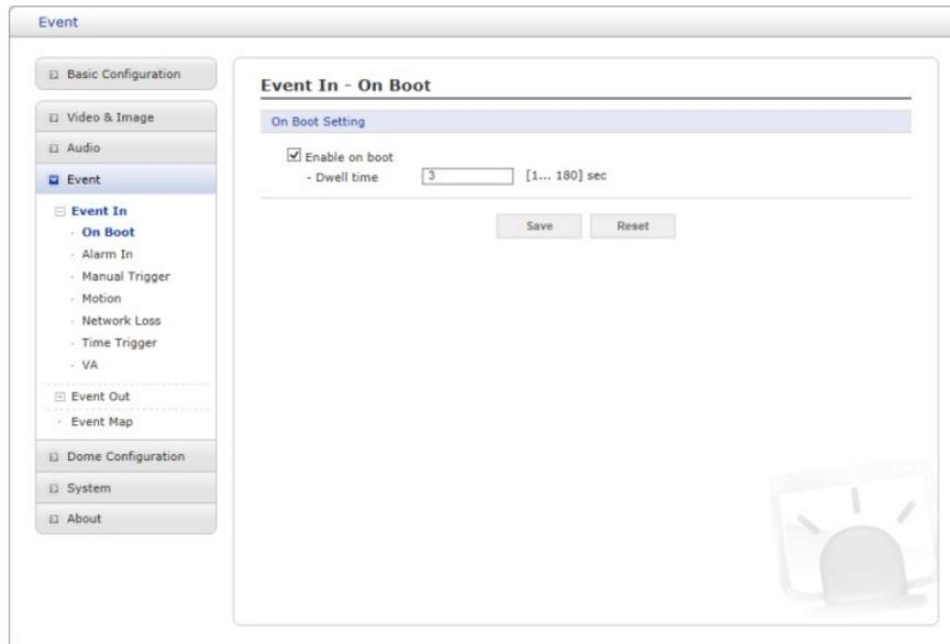
Trigger an event every time the camera is started. Select “Enable on boot” to activate. Enter the dwell time that the event lasts for from the point of detection, 1 ~ 180 seconds. Click ‘Save’ to save the settings, or click ‘Reset’ to clear all the changes.
