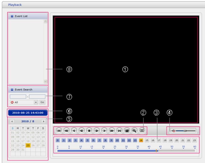
The Playback window contains a list of recordings made to the memory card. It shows each recording's start time, length, the event type used to start the recording, calendar and time-slice bar indicates if the recording exists or not.
