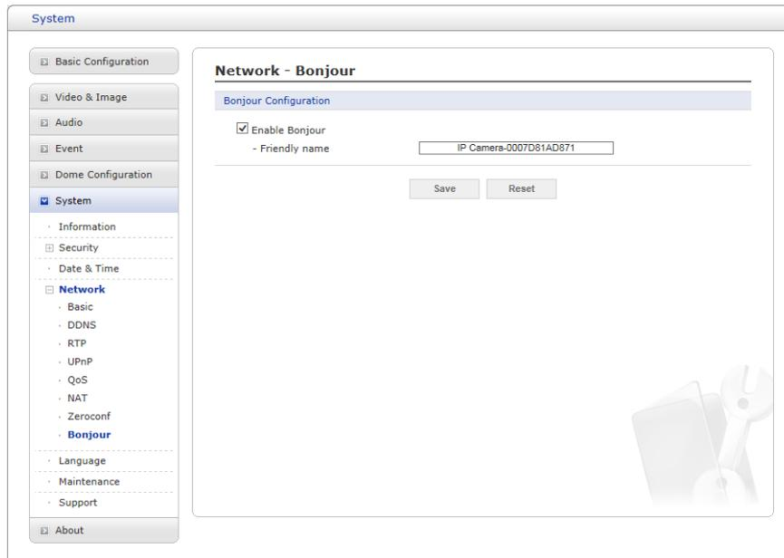
The camera includes support for Bonjour. When enabled, the camera is automatically detected by operating systems and clients that support this protocol.
