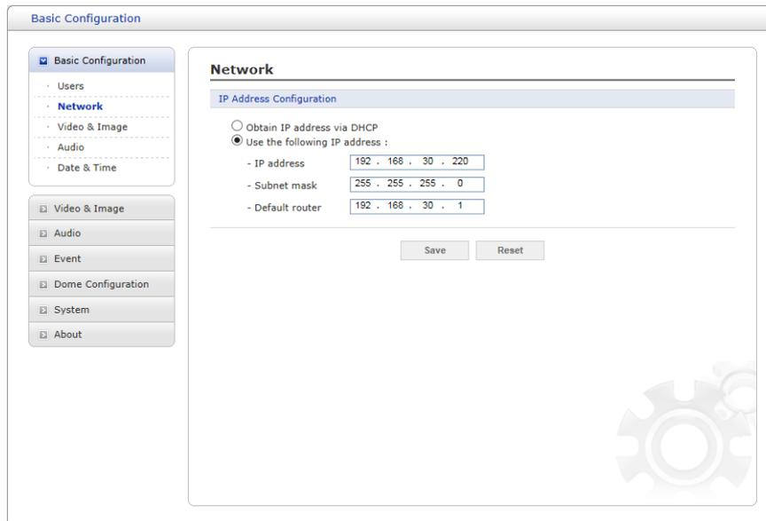
The screenshot shows the 'Basic Configuration' window with the 'Network' section selected. Under 'IP Address Configuration', the 'Use the following IP address' option is selected. The fields are filled with: IP address: 192.168.30.220, Subnet mask: 255.255.255.0, and Default router: 192.168.30.1. There are 'Save' and 'Reset' buttons at the bottom.
