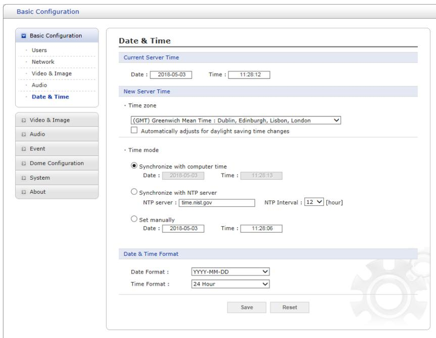
Users can set time directly or assign a time server to get the current time, as well as determine Date and Time format on this page.
