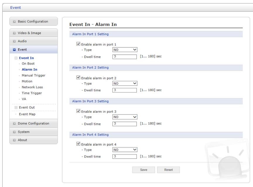
The camera has 4 alarm inputs. To use an alarm port, check the “Enable alarm port #” first.
