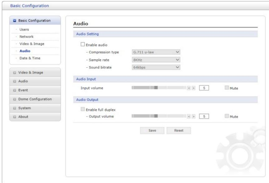
The camera can transmit audio to other clients using an external microphone and can play audio received from other clients by attaching a speaker. Users can setup and change the setting of Audio on this page.
