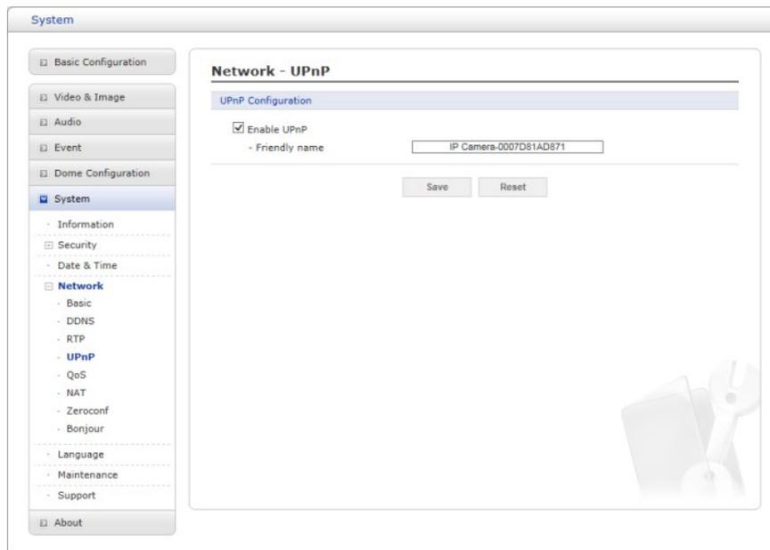
The camera includes support for UPnP. UPnP is enabled by default, so the camera is automatically detected by operating systems and clients that support this protocol.
