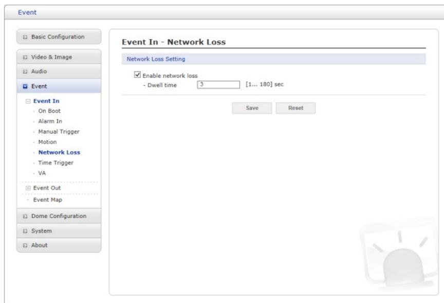
This is used to trigger an event every time the network connection fails. Select “Enable network loss” to activate the Network Loss event trigger. Select a dwell time for how long the event will last from the point of detection.
