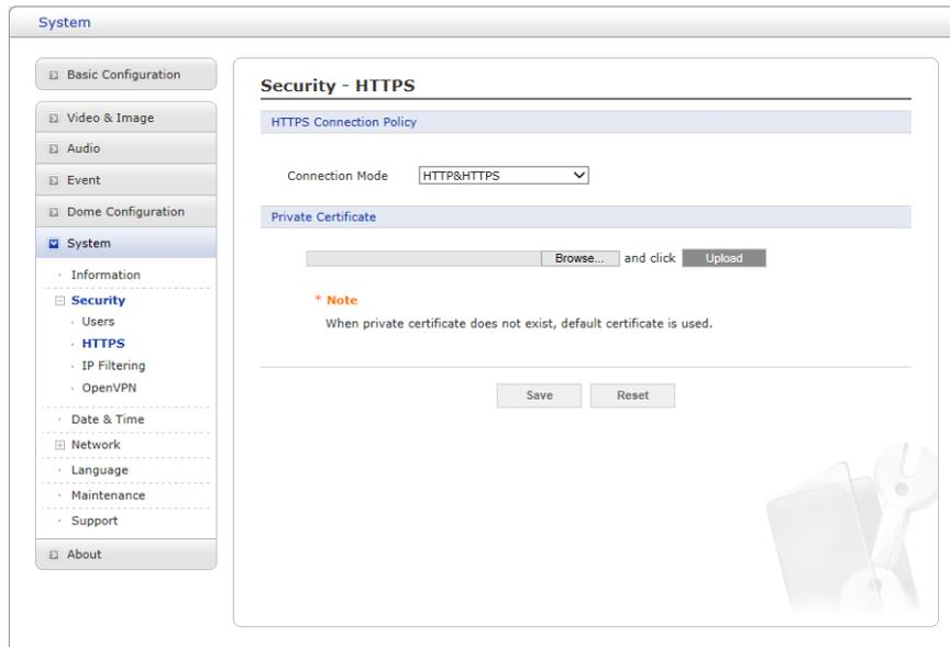
For greater security, the camera can be configured to use HTTPS (Hypertext Transfer Protocol over SSL (Secure Socket Layer)). All communication that would otherwise go via HTTP will instead go via an encrypted HTTPS connection.
