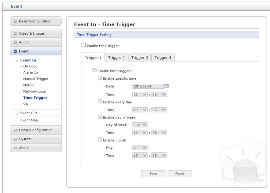
Time Trigger may be used to set alarms at a specific time. Users can set up to four time triggers. Each time trigger can be set to a specific date in the calendar, everyday, a day of the week, or the same date every month.
