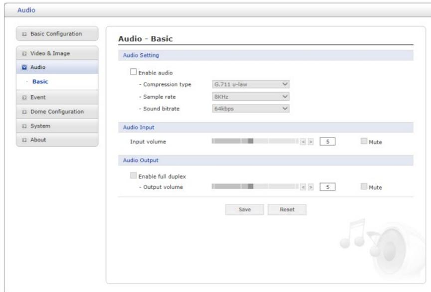
The camera can transmit audio to other clients when using an external microphone and can play audio received from other clients when using an attached speaker. The Setup page has an additional menu item called Audio, which allows different audio configurations, such as full-duplex and simplex.
