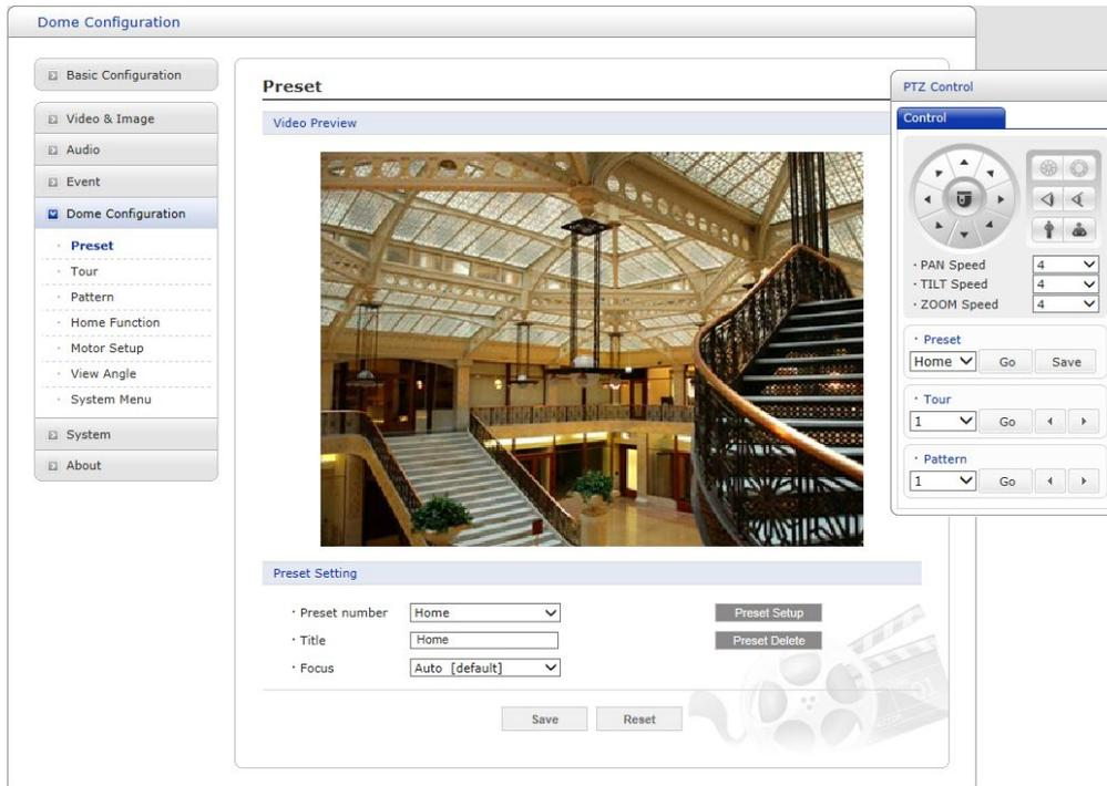
If you need to view specific places routinely, you should program Presets. A Preset is a programmed video scene with automatic pan, tilt, zoom, and focus settings. Once programmed, clicking the Preset number or clicking the Go button in the PTZ Control Panel calls up that Preset automatically.
