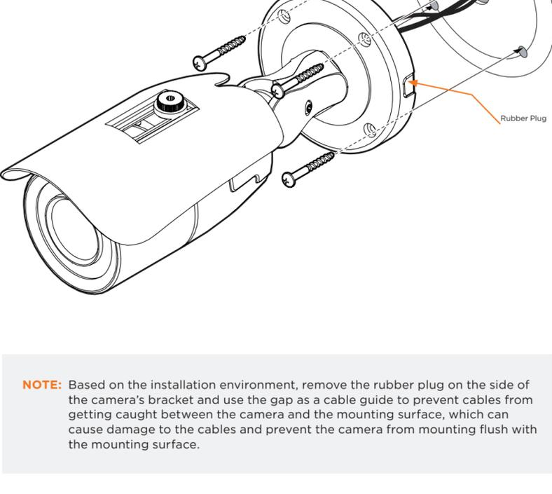
**NOTE:** Based on the installation environment, remove the rubber plug on the side of the camera's bracket and use the gap as a cable guide to prevent cables from getting caught between the camera and the mounting surface, which can cause damage to the cables and prevent the camera from mounting flush with the mounting surface.
