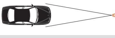
THE CAMERA SHOULD BE MOUNTED AT AN ANGLE NO GREATER THAN 30 DEGREES
