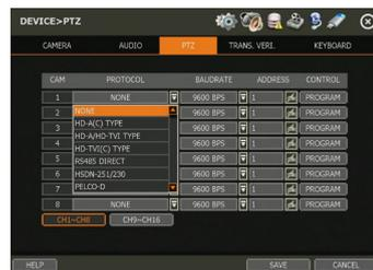
2. Camera type will be auto-detected and displayed under the camera tab. Protocol should match the camera type detected.
