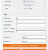
'Port forwarding' has to be set in your network's router for external access to the camera.
