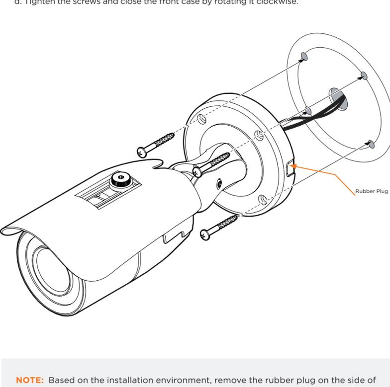
**NOTE:** Based on the installation environment, remove the rubber plug on the side of the camera's bracket and use the gap as a cable guide to prevent cables from getting caught between the camera and the mounting surface, which can cause damage to the cables and prevent the camera from mounting flush with the mounting surface.
