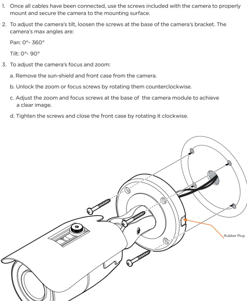
**NOTE:** Based on the installation environment, remove the rubber plug on the side of the camera's bracket and use the gap as a cable guide to prevent cables from getting caught between the camera and the mounting surface, which can cause damage to the cables and prevent the camera from mounting flush with the mounting surface.
